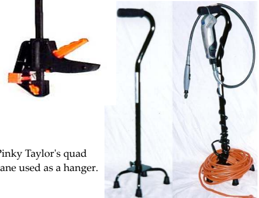
Clamping hanger - with a closeup of the squeeze trigger clamp mechanism.
