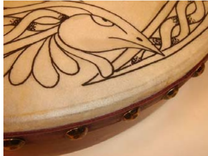
The skin is stapled on while damp. A leather strip and decorative nails hide the staples.
